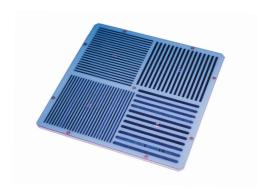
Four-quadrant bar phantoms offer precise determination of camera intrinsic resolution, collimator spatial resolution, field size and linearity.
